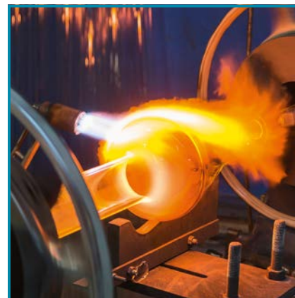
Glass tubes are blown by highly skilled blowers to ensure the uniform wall thickness, exact dimensions according to DIN standards.
