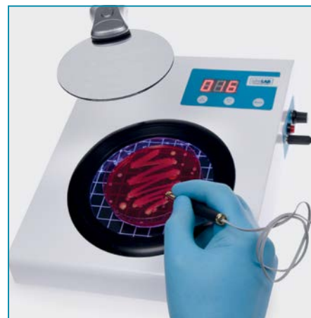
Marking is done by a "felt pin pen" which is connected to the system by cable.
