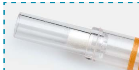
Filter plug at the mouthpiece prevents overflow of liquid and also eliminates contamination.
