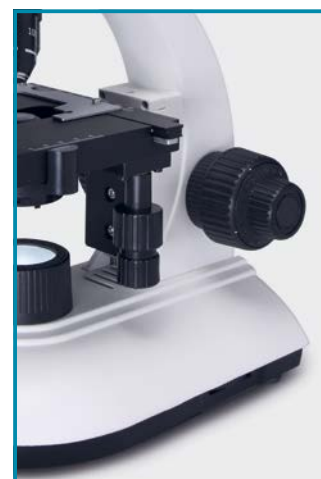
Coarse and fine adjustment is enabled with upper limit safety with 0,002 mm fine division and 20 mm moving limit. Each rotation of control knob enables 42,4 mm coarse stroke and 0,2 mm fine stroke.
