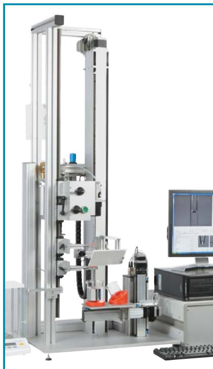
Steps such as filling the water, finding the meniscus line and controlling the volume are done automatically.
