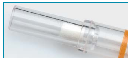
Filter plug at the mouthpiece of the pipette prevents exterior effects and minimize contamination.
