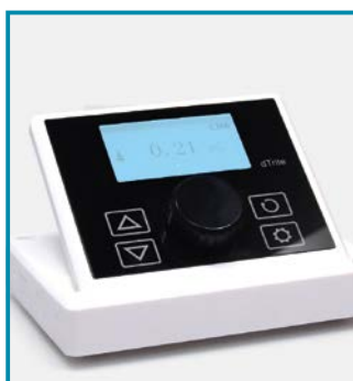
TFT control touchscreen guides the user for a quick and accurate titration.
