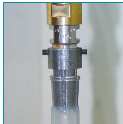
Grinding steps are performed by diamond reamers assuring best results with highest precision.
